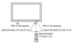
Other devices which use infrared beams, sunlight, fluorescent lights, etc., may affect the range and effectiveness of the remote control. Make sure the plasma display is positioned in a place which minimizes interference from them.
